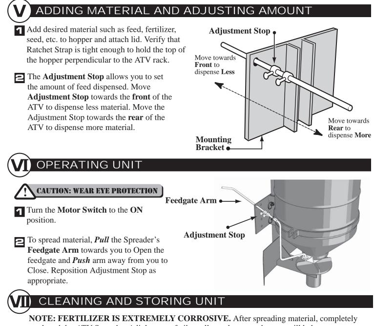
**NOTE: FERTILIZER IS EXTREMELY CORROSIVE.** After spreading material, completely wash and dry ATV Spreader. A light coat of oil on all metal parts and motor will help prevent rusting and corrosion.
