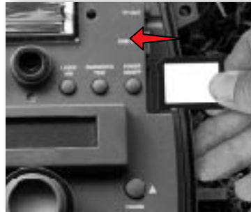
SD MEMORY CARD CAPACITY Maximum card size allowed is 256 MB (sold separately)
