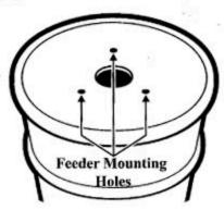
1 From the inside of the drum, slide the three provided Bolts through the holes on the bottom and into the provided Flat Nuts. From the inside, using a Phillips head screwdriver, turn the Bolt clockwise until the Flat Nut is tight against the bottom.
