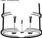
Slide feeder over three Bolts that are sticking firmly through the bottom of the drum. Attach Feeder to the Drum using the three provided Wing-Nuts.
