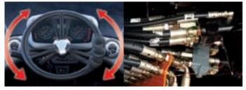
**Hydraulic Power Steering** The newly designed steering system ensures smooth steering even in the low engine speed ranges.
