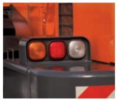
**Rear combination lamp** A semi-permanent lamp life has been secured with the application of LED-type stop and position lamps.
