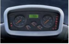
**Central indicator panel** A high visibility indicator panel allows the operator to check essential loader functions.
