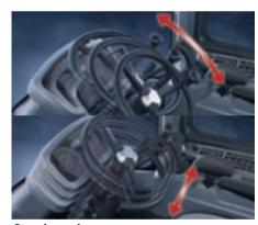
**Steering column** The steering column features both tilting and telescopic functions.
