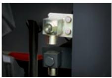
**Engine oil and coolant drains** Drains are installed in very accessible places to facilitate emptying without the risk of polluting the environment.
