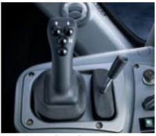
**Control levers (option)** The control levers are very precise. Different options are available to match what the operator is accustomed to as well as an optional auxiliary lever.
