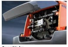
**Reversible fan** The radiator fan has a reversible flow capability to make cleaning of the coolers easier when the machine is operating in dusty environments.
