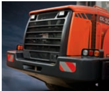
Radiator Grill (Steel structure)
