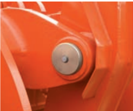
Covering(On pin-end) Pin & Bush Improved
