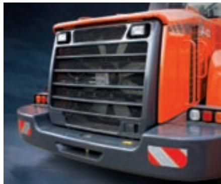
Radiator Grill (Steel structure)
