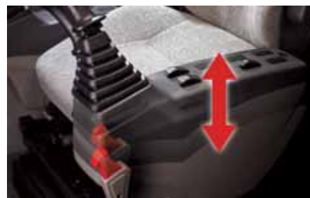
Control stand (Telescopic Function)
