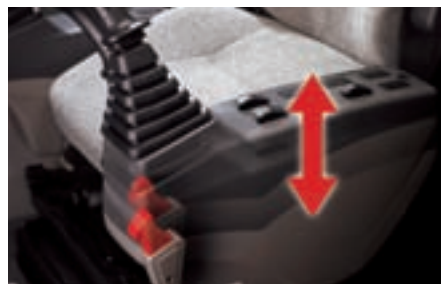
Control stand (Telescopic Function)
