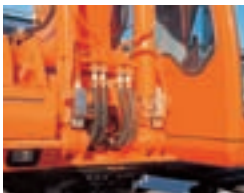
Boom and arm hose rupture protection valve
