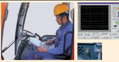
By connecting a laptop PC to the controller (e-EPOS controller) of the machine, data such as pump pressure and engine RPM can be displayed graphically. Also other various machine status data can be stored in memory and printed out using a printer.
