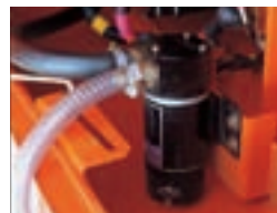
Electric fuel supply pump
