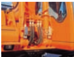
Boom and arm hose rupture protection valve
