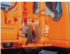
Boom and arm hose rupture protection valve
