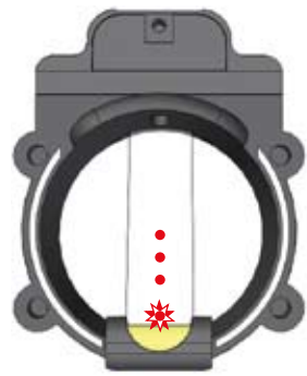
Pin will be at bottom off screen - Press (-) to bring it up one position.
