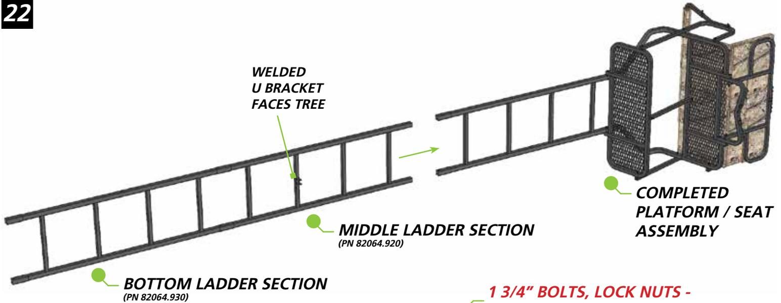
**1 3/4" BOLTS, LOCK NUTS - WRENCH TIGHTEN**
