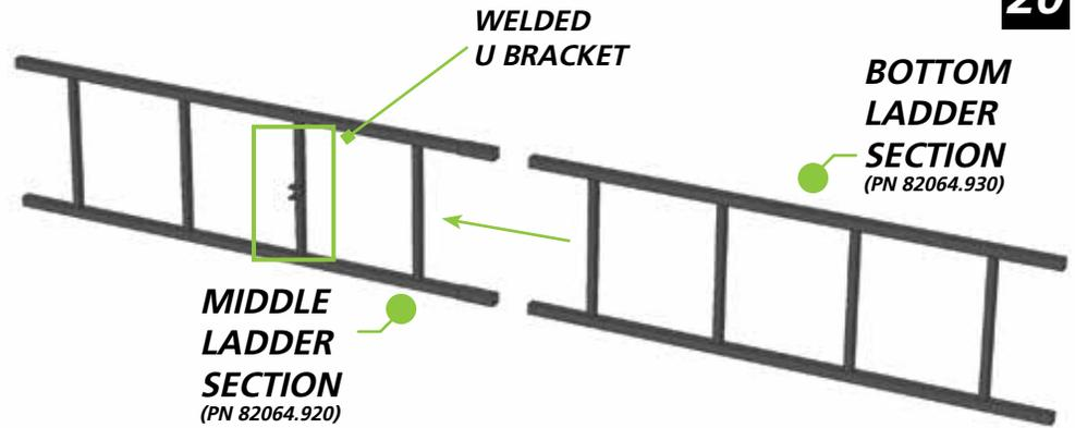
**1 3/4" BOLTS, LOCK NUTS - WRENCH TIGHTEN**
