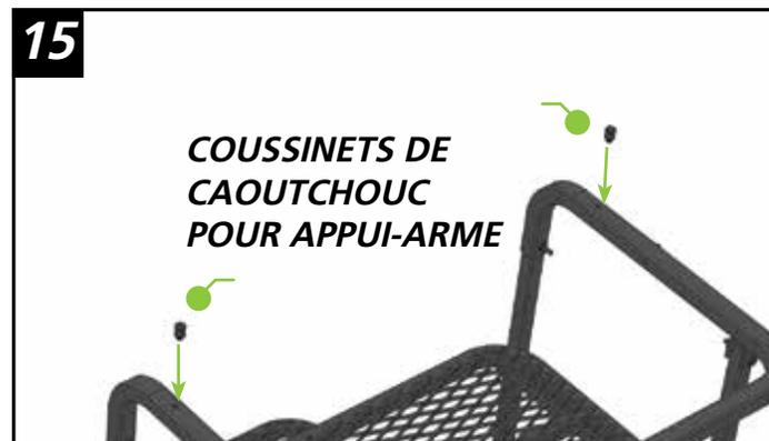
COUSSINETS DE CAOUTCHOUC POUR APPUI-ARME
