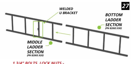
1 3/4" BOLTS, LOCK NUTS WRENCH TIGHTEN
