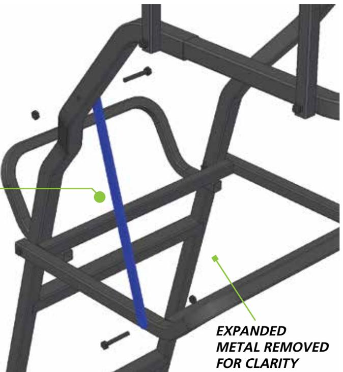
**1 3/4" BOLTS, LOCK NUTS - WRENCH TIGHTEN STEP 9**
