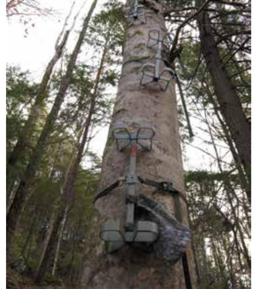
Summit recommends the use of the Seat-O-The-Pants Climbing system (PN 83014 or 83024) for any Hang-On stand. After hooking the SOP Climbing System to the tree you can climb and stay connected directly to your safety harness at all times.
