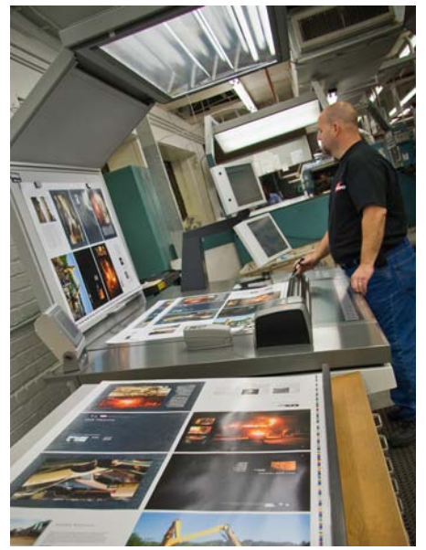
All operations of the press are controlled by the operator at the main terminal.
