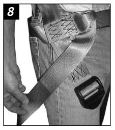
**4.** Thread leg strap through leg buckle as shown in *figure 9*. Pull tag end of leg strap to adjust fit as shown in *figure 10*. Leg strap should be comfortably snug (see *figure 11*). Pull the tag end of the leg strap back through the buckle as shown in *figure 12* and in f*igure 13*.
