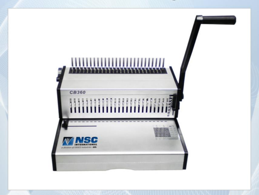
The NSC CB360 is a traditional plastic comb punch and bind machine in appearance, but takes performance to a higher level. With all metal construction and 24 hardened steel punching dies that easily punch 25 sheets of paper, the CB360 can bind books up to 2" (50 mm), approximately 450 pages, and up to legal size (14") in length. For consistent binding needs in moderate volume, there is no better value in today's binding market.
