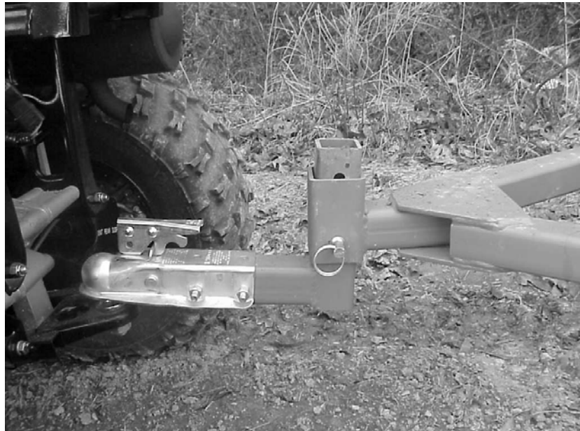
Figure 6: The Plot Mule also has an adjustable coupler to allow adjustment height of the coupler to your specific ATV. Adjust the coupler with the wheels up and disc setting on the ground. This must be adjusted to equally distribute the cutting action between the front and rear gangs.
