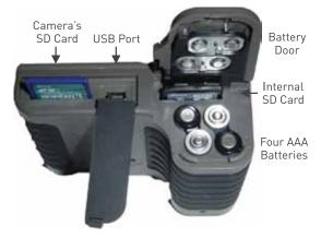
The maximum capacity of the SD card is 16GB. It is recommended that the Internal SD Card have larger capacity than the camera's SD Card, since the **Internal SD** is used to store images that are transferred from the camera's SD Card.
