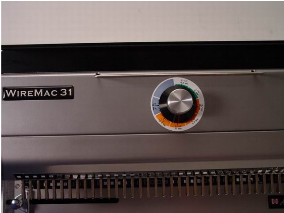
Wire Closer Selector: Gradual adjustment ensures a secure closure every time.
