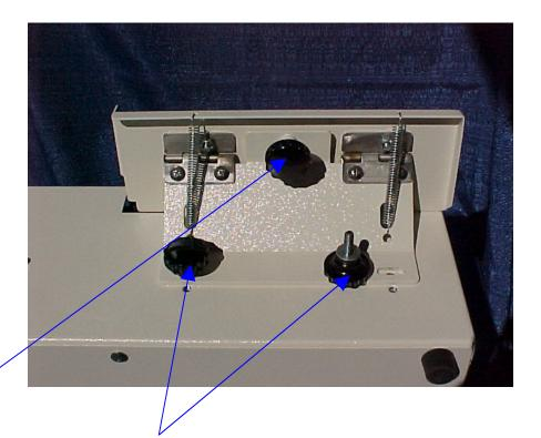
The worktable is fastened to the crimper using the ¼" stud knobs and two ¼" flat washers included with your machine. The holes in the table are slotted allowing side to side adjustments to be made. Mount the table in the top holes for small and medium diameter coil and the bottom holes for medium and large diameter coil.
