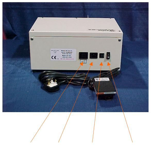
Foot Pedal AC power cord ½ Amp fuse power switch
