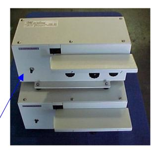
**Plunger Switch:** Only models produced for sale in the USA will come with plunger switch. An optional foot pedal can be purchased.
