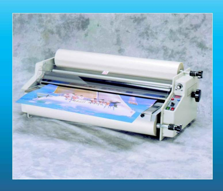
film have been run through the machine, bottom idler threading is automatic when the operator puts the feed tray on the machine.
