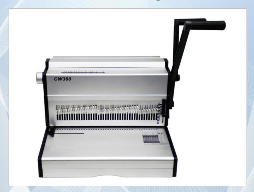
The CW360 is a heavy duty manual punch and closing unit for double loop wire in the popular 3:1 pattern. The CW360 is ideal for any document finishing environment with consistent binding needs. All metal construction and attractive design ensures that the CW360 is a rugged and durable performer for wire bound books up to 9/16" (14mm) in diameter.
