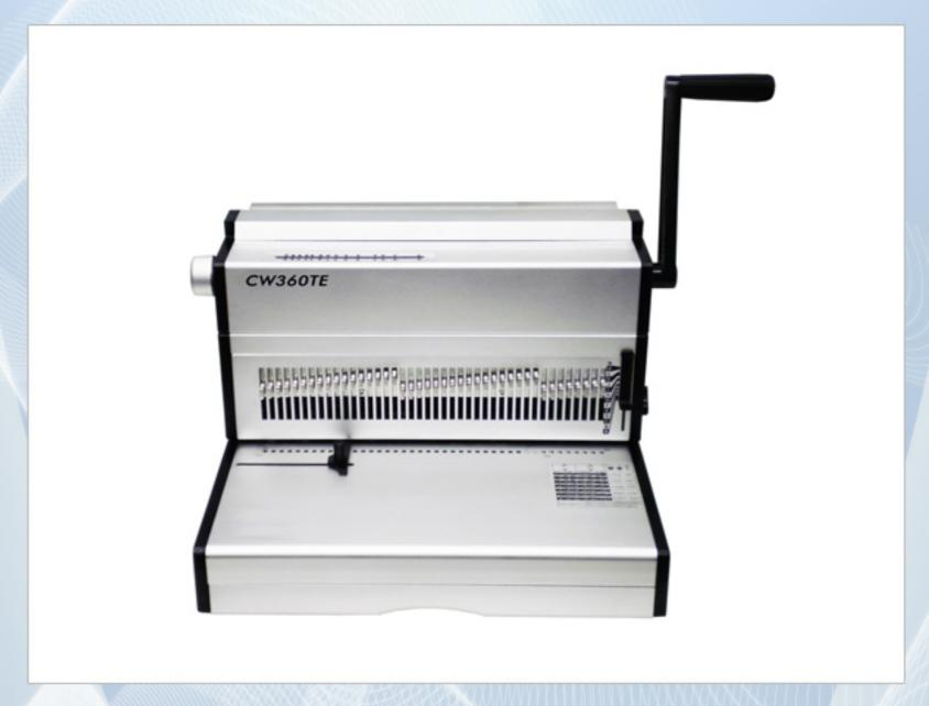
The CW360TE is a heavy duty electric punching unit with closer for double loop wire in the popular 2:1 pattern. The CW360TE is ideal for any document finishing environment with consistent binding needs. All metal construction and attractive design ensures that the CW360TE is a rugged and durable performer for wire bound books up to 1 1/4" (32mm) in diameter.
