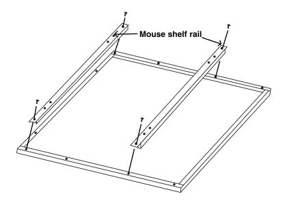
Attach the mouse shelf support bars to the first holes and third holes on the bottom of the keyboard shelf with 4-sheet screws. Then align the brackets on the mouse shelf to the holes on the support bars and attach using 8 sheet metal screws.
