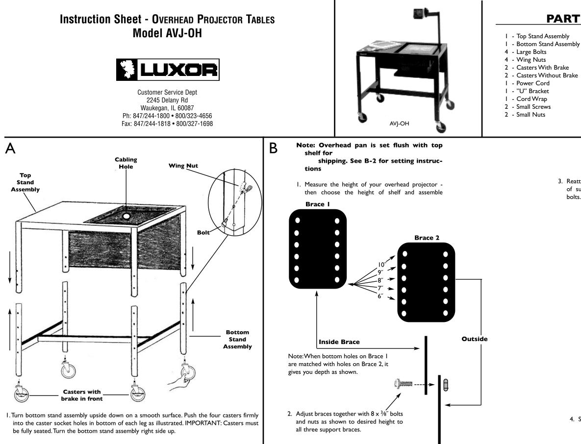
2. Position top stand assembly over bottom stand assembly as illustrated. Adjust top stand assembly up or down to desired height. Align holes in all four legs, insert bolts and fasten with four wing nuts as illustrated.
