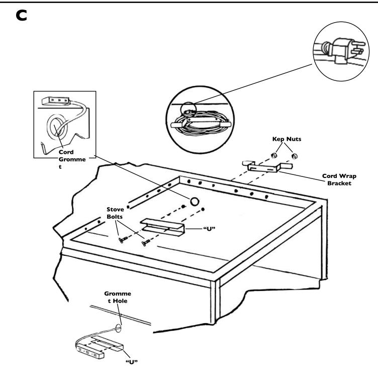
Press 3-outlet power cord into "U" bracket and feed remaining cord through grommet hole and wrap remaining cord around cord wrap bracket. For safety and neat appearance, secure plug to cord with plug snap.
