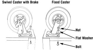
Turn your equipment table upside down. Install the two swivel casters on the end of the table with the handle using 8 bolts, flat washers and nuts.
