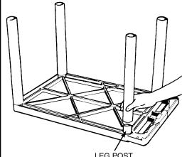
2. Lay top shelf (with handle) ribbed side up on a smooth surface. Push all 4 legs onto leg posts.
