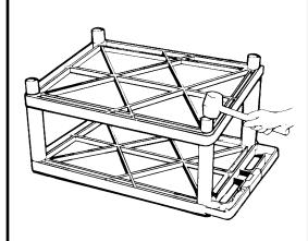
2. Position center shelf (with 8 leg posts) ribbed side up over the 4 legs and insert leg posts into short legs. Using a rubber mallet, firmly hammer center shelf into legs until all four legs are seated (flush) against the surfaces of both shelves.
