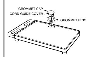
1. Install grommet ring by tapping into place with rubber mallet. Insert grommet cap as illustrated. For tables with electric assembly, snap off cord guide cover from grommet cap so equipment plug may be run through grommet to plug unit. Then insert grommet cap into grommet ring.
