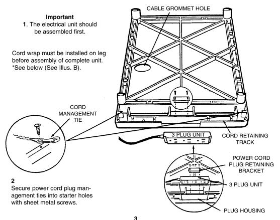
Firmly seat electric assembly 3 plug unit into handle plug housing as illustrated. Secure with power cord plug retaining bracket.
