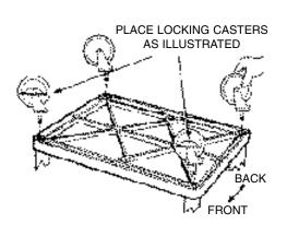
**5.** Push the four casters firmly into the holes in each corner of the bottom shelf. Important: Casters must be fully seated. Tap firmly with rubber mallet to properly seat casters. Turn your Endura Table right
