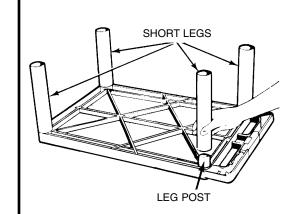
1. Install grommet ring and cap as illustrated in Step #1 above. Lay top shelf (with handle) ribbed side up on a smooth surface. Push all 4 short legs onto leg posts.
