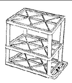
4. Position bottom shelf, ribbed side up, over the 4 long legs and insert leg posts into long legs. Firmly hammer bottom shelf until seated onto all 4 legs.
