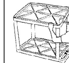
3. Position bottom shelf, ribbed side up, over the 4 legs and insert leg posts into legs. Using a rubber mallet, firmly hammer bottom shelf into legs until all four legs are seated (flush) against the surfaces of both shelves.
