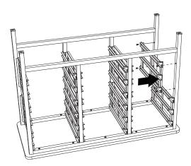
Step 2: Screw Certwood rails to the legs with M6 x 10 Flat Phillips screws.
