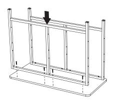
Step 1: Screw legs to top with the M6 x 35 Allen Screws.
