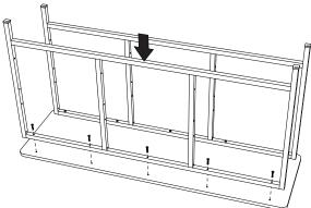
Step 1: Screw legs to top with the M6 x 35 Allen Screws.
