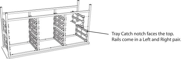
Step 2: Screw Certwood rails to the legs with M6 x 10 Flat Phillips screws.
