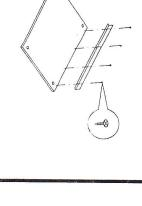
Install shelf support brace to the left and right side panels using 4 - 1 1/2" allen head screws.
