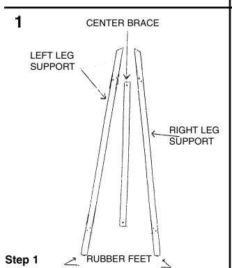
Lay the left leg, the right leg, and center brace on the ground with the pre drilled holes facing up. Then attach the top support brace and bottom support brace using 11/2" wood screws. Note: You will use all 10 11/2" screws for this step.
