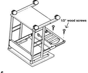
Step 6 Align the four predrilled holes on the bottom of the keyboard corners and attach with the 4-1/2" wood screws.
