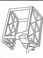
Position bottom shelf, ribbed side up, over the 4 legs and insert leg posts into legs. Using a rubber mallet, firmly hammer bottom shelf into legs until all four legs are seated (flush) against the surfaces of both shelves. 4. Push the four casters firmly into the holes in each corner of the bottom shell. Important: Casters must be fully seated. Tap firmly with rubber mallet to property seat casters. Turn your Endura Table right side up.
