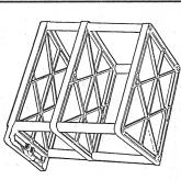
4. Position bottom shelf, ribbed side up, over the 4 long legs and insert leg posts into long legs. Firmly hammer bottom shelf until seated onto all 4 legs.
