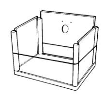
Install the back panel in the same manner as shown in Step #3. NOTE: Cabling hole in back panel should be toward the top.
