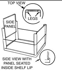
Install the side panels first. Slide panels down between legs until they are nested inside the shelf lip and flush against the shelf surface. Rubber band will hold legs and side panels in place while installing back panel and front door.
