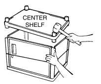
Begin seating of center shelf by holding door panel, leg and side panel as illustrated. Gently tap corner post into leg. Repeat on all 4 sides until all posts are partially inserted into legs. Now repeat hammering action more firmly going around to each shelf post and driving the leg posts more securely into the legs.
