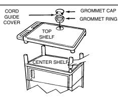
Push remaining 4 legs onto center shelf posts as illustrated. Place top shelf (with handle) onto legs. Insert leg posts into legs of top shelf. Úsing rubber mallet, firmly hammer top shelf into legs until all four legs are seated against shelf surface. install grommet ring and grommet cap into top of shelf. For tables with electric assembly, snap off cord guide cover form grommet cap to allow equipment plug to be run through grommet. Insert grommet cap into grommet ring. Remove rubber band.
