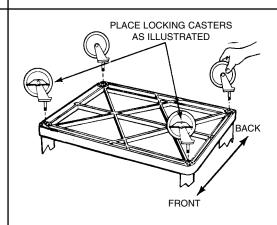
Push the four casters firmly into the holes in each corner of the bottom shelf. Important: casters must be fully seated. Tap firmly with rubber mallet to properly seat casters. Turn your Endura Table right side up.
