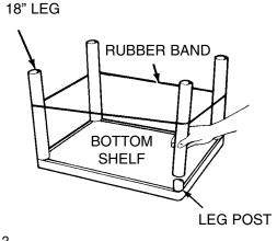
With bottom shelf facing up push all four 18" legs onto leg posts. Using rubber mallet hammer legs firmly into position. Legs must be seated (flush) against the shelf surface. Place rubber band around legs to aid in the assembly of cabinet side panels and doors
