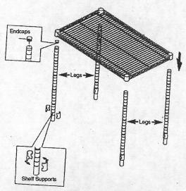
1. Install shelf supports onto the lowest grooves of the legs. Insert leg end caps into the top of legs. Slide legs through the corners of one shelf and fully seat onto plastic shelf suports.
