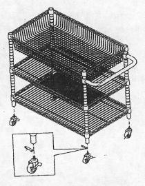
Turn cart onto it's side and install the casters. Be sure the two casters with brake are on the same side. Tighten with wrench.
