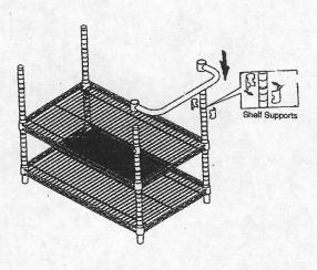
2. Install second batch of shelf supports onto legs to desired height of the middle shelf, and install shelf. Attach 2-sets of shelf supports to either side of the cart, and slide handle onto shelf supports.
