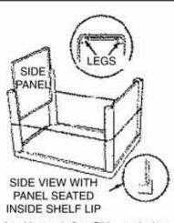
Install the side panels first. Slide panels down between legs until they are nested inside the shelf lip and flush against the shelf surface. Rubber band will hold legs and side panels in place while installing back panel and front door.
