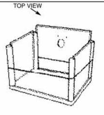
Install the back panel in the same manner as shown in Step #3. NOTE: Cabling hole in back panel should be toward the top.
