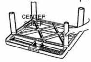
Begin seating of center shelf by holding door panel, leg and side panel as illustrated. Gently tap corner post into leg. Repeat on all 4 sides until all posts are partially inserted into legs. Now repeat hammering action more firmly going around to each shelf post and driving the leg posts more securely into the leas.
