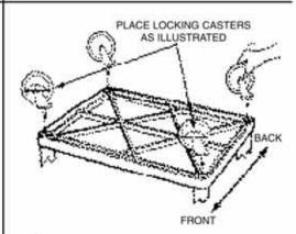
Push the four casters firmly into the holes in each corner of the bottom shelf. Important: casters must be fully seated. Tap firmly with rubber mallet to properly seat casters. Turn your Endura Table right side up.
