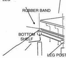
With bottom shelf facing up push all four 18" legs onto leg posts. Using rubber mallet hammer legs firmly into position. Legs must be seated (flush) against the shelf surface. Place rubber band around legs to aid in the assembly of cabinet side panels and doors.
