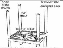
Place top shelf (with handle) onto legs. Insert leg posts into legs of top shelf. Using rubber mallet, firmly hammer top shelf into legs until all four legs are seated against shelf surface, install grommet ring and grommet cap into top of shelf. For tables with electric assembly, snap off cord guide cover form grommet cap to allow equipment plug to be run through grommet. Insert grommet cap into grommet ring. Remove rubber band.
