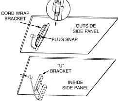
Press 3-outlet power cord into "U" bracket and feed remaining cord through grommet hole and wrap remaining cord around cord wrap bracket. For safety and neat appearance, secure cord plug to cord with plug snap.
