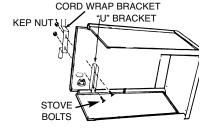
Insert two stove bolts as illustrated through "U" bracket into side panel and through slots in cord wrap bracket. Align the cord wrap bracket onto machine screws from the outside of back shelf and secure with two kep nuts.
