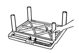
Lay top shelf (with handle) ribbed side up on a smooth surface. Push all 4 short legs onto leg posts.
