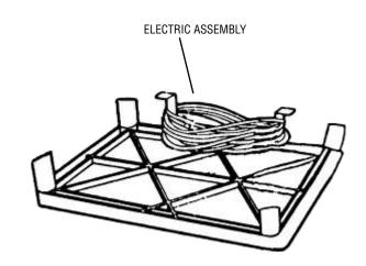
Align cord bracket to the pre-drilled holes on the underside of the middle and attach using two silver screws.
