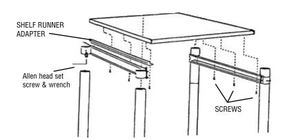
Slide runners onto the legs and tighten down to desired height. Align holes on the shelf adapters to the holes on the bottom of the keyboard and attach using six sheet metal screws. Slide the rear of the shelf adapters under the tab on the back of the runners and snap the front of the shelf adapters onto the back tongue on the front of runners.
