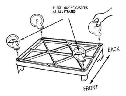
Push the four casters firmly into the holes in each corner of the bottom shelf. Important: casters must be fully seated. Tap firmly with rubber mallet to properly seat casters.
