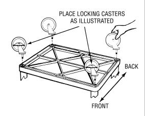
Push the four casters firmly into the holes in each corner of the bottom shelf. Important: casters must be fully seated. Tap firmly with rubber mallet to properly seat casters. Turn your table right side up. It is now ready for use.
