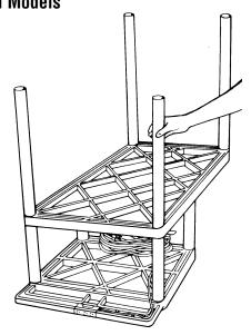
Push set of 4 long legs into leg posts of second shelf and firmly hammer until properly seated
