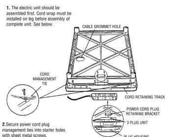
3. Firmly seat electric assembly 3 plug unit into handle plug housing as illustrated. Secure with power cord plug retaining bracket.
