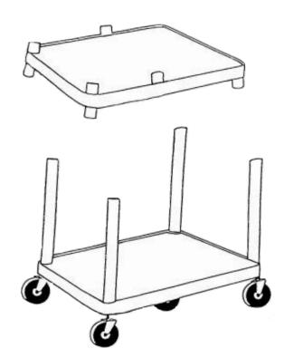
Insert longer legs onto the leg post on the bottom shelf and firmly hammer until properly seated. Then insert the leg post on the middle shelf into the legs.
