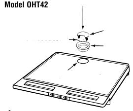
Install grommet ring by tapping into place with rubber mallet. Insert grommet cap as illustrated. For tables with electric assembly, snap off cord guide cover from grommet cap so equipment plug may be run through grommet plug unit, then insert grommet cap into grommet ring.
