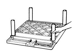
Lay top utility shelf (with handle) ribbed side up on a smooth surface. Push all 4 short legs onto leg posts.
