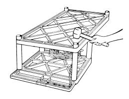
Position second shelf (with 8 leg posts) ribbed side up, over the 4 legs and insert leg posts into legs. Using a rubber mallet, firmly hammer bottom shelf into legs until all four legs are seated (flush) against the surfaces of both shelves.
