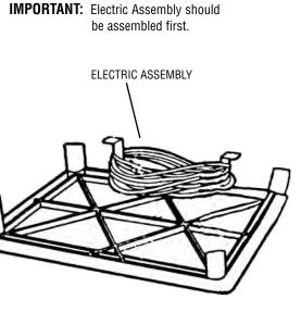
Align cord bracket to the pre-drilled holes on the underside of the middle and attach using two silver screws.
