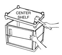
6 Begin seating of center shelf by holding door panel, leg and side panel as illustrated. Gently tap corner post into leg. Repeat on all 4 sides until all posts are partially inserted into legs. Now repeat hammering action more firmly going around to each shelf post and driving the leg posts more securely into the legs. Top of panels and door frame must be nested into the underside of the center shelf lip in the same manner as the bottom shelf.
