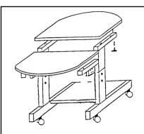
3. Attach keyboard shelf and monitor shelf to base assembly using 2 3/8" flat head screws, 4 per shelf.
