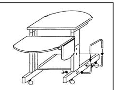
6. Install CPU holder on right or left side of workstation. Install nut and washer on silver 'L" support. Put threaded end of 'L" support through lower section of leg. Install plastic spacer and nut on inside of leg. Using the threaded portion of the "L", adjust for width of CPU by moving nuts. Slide upper portion of CPU holder over two silver "L" supports.
