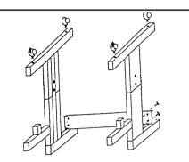
1. Screw casters into left and right leg assembly positioning casters with brake towards the front. Screw rear support panel onto back of left and right leg assembly, using 4 9/16" flat head screws. Use two phillips head screws and matching nuts to attach "U" bracket to rear support panel. The heads of the phillips head screws should be inside the "U" bracket.
