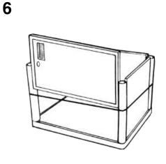
Install door panel same as back panel with door handle at top. Be sure door opens outward and door frame is also placed between legs and nested flush on the shelf floor.
