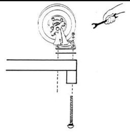
Bolt goes through shelf, through bracket, through caster plate, then is secured using kep nuts.
