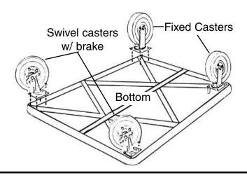
Check tire pressure every 30 days. Pressure should be maintained at 50 lbs.
