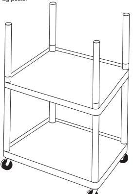
Slide the plastic cord wrap onto rear leg. Slide the runners onto the legs and tighten down to desired height with 4 allen head screws provided.
