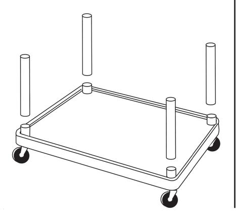
Insert leg post on the middle shelf into legs attached to the bottom shelf. Then insert longer legs onto middle shelf leg posts.
