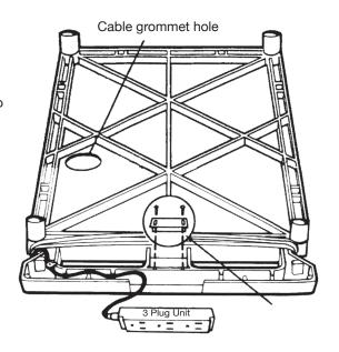
Keyboard shelf assembly—lay metal keyboard shelf on a flat surface so underside with holes is facing up. Attach each shelf runner adapter with 3 1/2" black Phillips head screws to each side of keyboard shelf.
