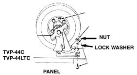
Bolt goes through hole in cabinet panel first, then through TVP unit then up through caster plate
